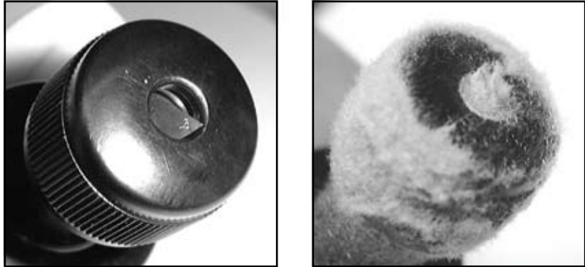
Figure 31. A clean blade holder (left) and a blade after cutting several sheets of twill (right).
